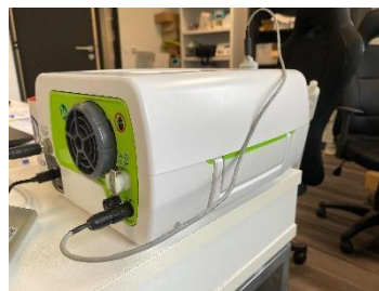
Figure 27: EO-150 ventilator connection to a (a) T-connector and (b) a FiO2 cell
