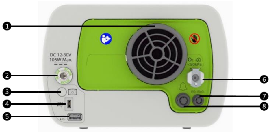
Figure 7: Rear view of the EO-150 ventilator and description of its features
