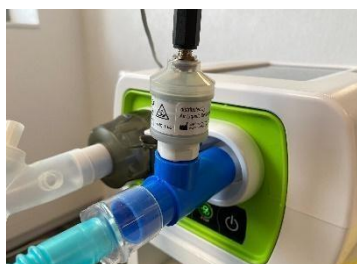
Figure 27: EO-150 ventilator connection to a (a) T-connector and (b) a FiO2 cell
